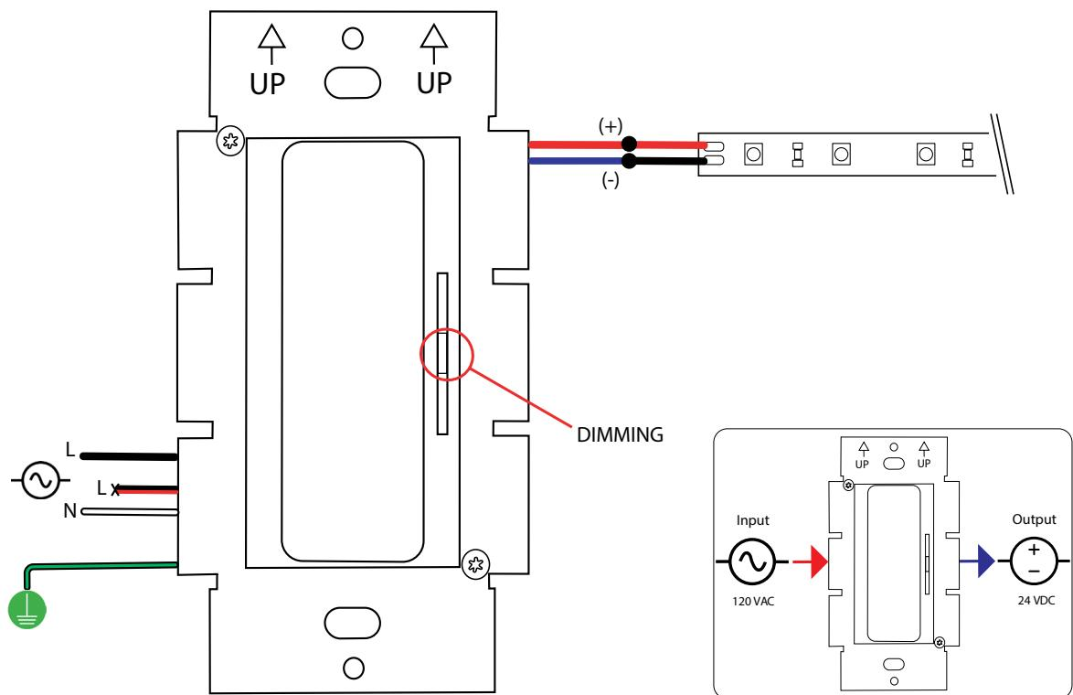
3-WAY DIMMING WIRING DIAGRAM
