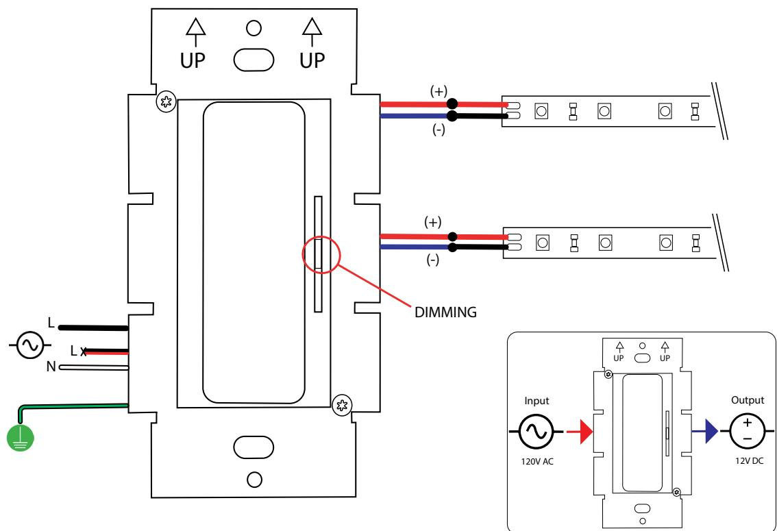
3-WAY DIMMING WIRING DIAGRAM
