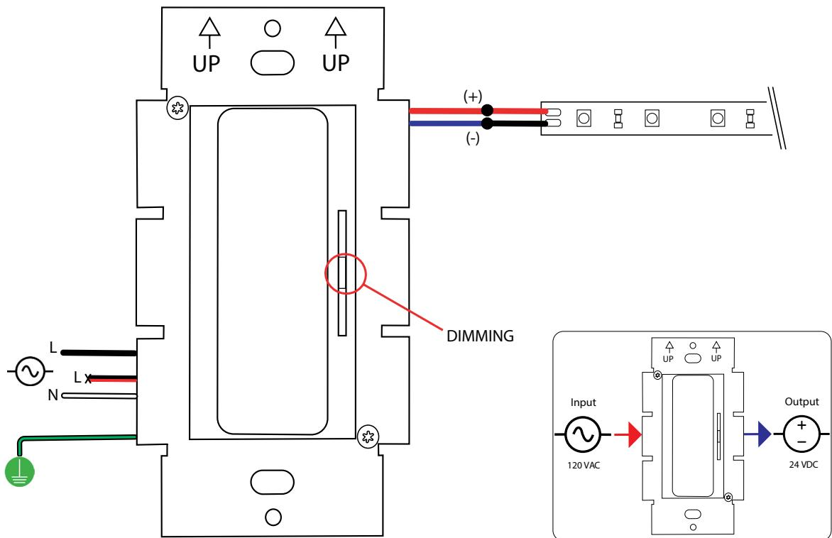
3-WAY DIMMING WIRING DIAGRAM
