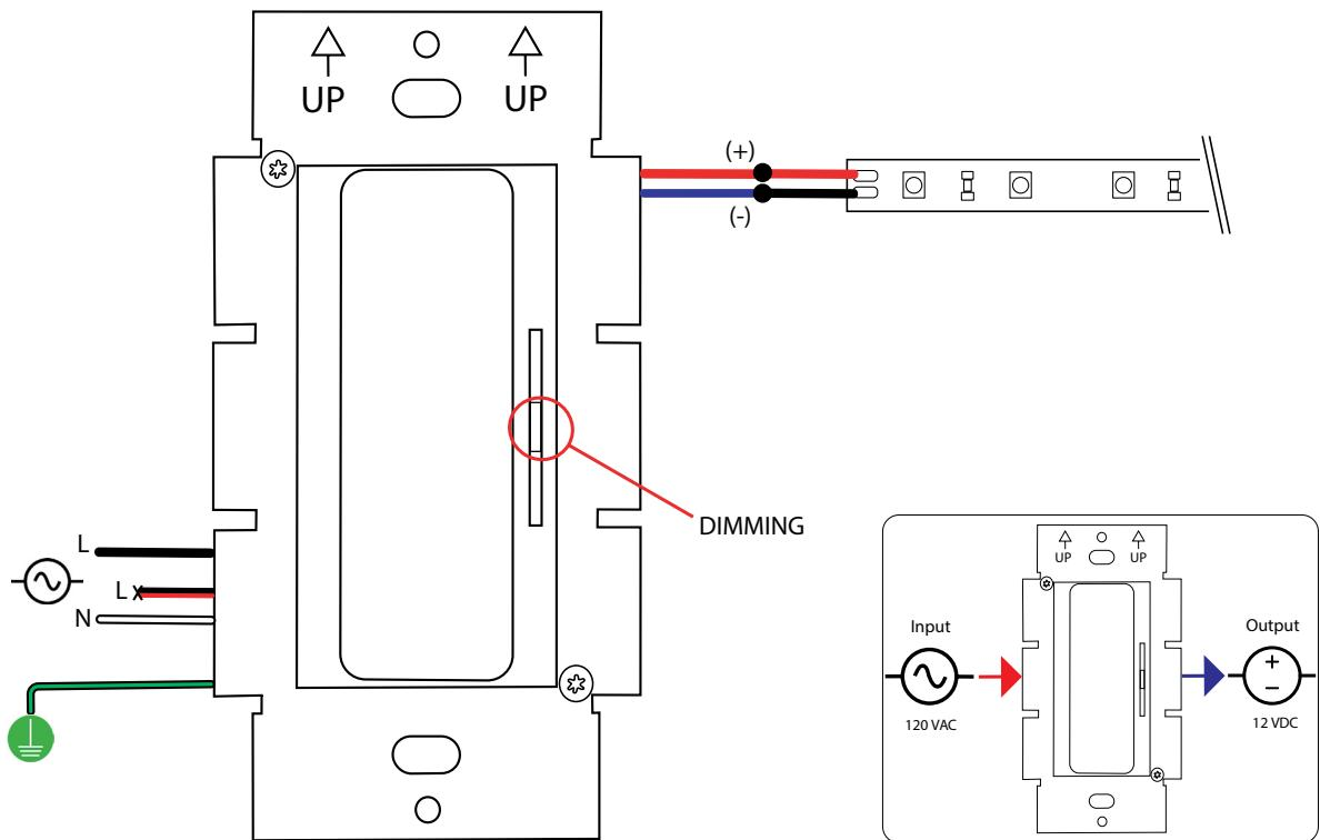
3-WAY DIMMING WIRING DIAGRAM
