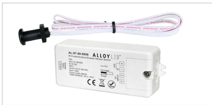
Our IR Proximity Door/Drawer Sensor Switch easily turns lights on automatically when you open a cabinet, drawer, closet, safe, or any other similarly darkened space. The Infrared (IR) sensor switch works on a DC input and is compact. The sensor will turn the lights on when the 6-cm (2 3/8 in.) beam is no longer interrupted. When you open your cabinet door or drawer, your lights will turn on and stay on for as long as the door remains open.
