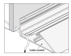
7. Pass the DC power cable through the 1/4 in. hole on the back into the cable conduit.
