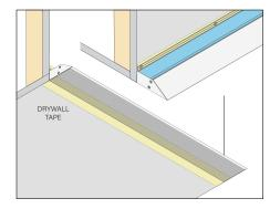
14. Apply drywall tape along the edges of the fixture to prevent the joint compound from cracking after installation, and smooth the tape flush.
