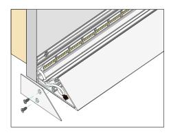
11. Assemble each end cap at the ends of Surfa KnifeEdge with two flat head screws provided.
