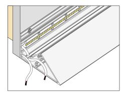
9. Remove the adhesive backing from the back of the LED tape. Apply the tape where shown. Pass the lead wire through the 11/64 in. hole into the cable conduit.
