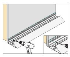
4. Drill 3/16 in. mounting holes along the drill port in the fixture to match the stud locations in the wall. Deburr any sharp edges.
