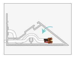
10. Connect LED tape lead to low-voltage in-wall rated wire. Red is positive (+) and black is negative (-). Place the wires in the cable conduit.
