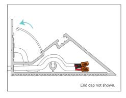
12. Test that the LEDs are working correctly before proceeding, then install the LED diffuser.
