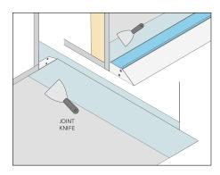
15. Apply joint compound mud to the mud-in flanges with a joint knife, covering the flanges and screw heads, and smooth the mud joint.
