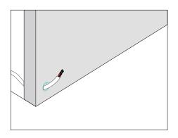
3. Bring power to a point through the wall that will match the position of the fixture's cable conduit.
