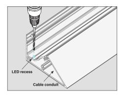
6. Drill a 11/64 in. hole through the floor of the LED recess into the cable conduit to provide wire access from the LED recess. Deburr any sharp edges.
