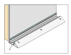
8. Place the fixture against the drywall panel and secure it with standard drywall screws into the 3/16 in. holes aligned with the stud locations in the wall.
