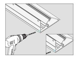
5. Drill a 1/4 in. hole through the back of the fixture this will be used for the power feed. Deburr any sharp edges.
