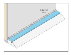
13. Cover the inside of the fixture with painter's tape if necessary before plastering, to prevent joint compound and dust from entering.
