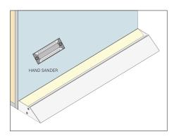
16. Once dry, use the hand sander to smooth the mud to make a seamless look with the drywall. Then remove the painter's tape.
